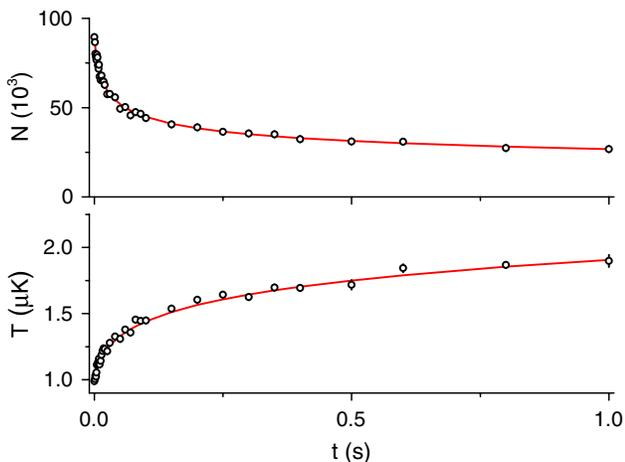
FIG. 1 (color online). Particle loss and heating in a resonantly interacting Bose gas ( $\lambda/a = 0$ ). Each point is an average of 5 measurements and error bars show standard statistical errors. Solid red lines are fits based on Eqs. (5) and (3).
