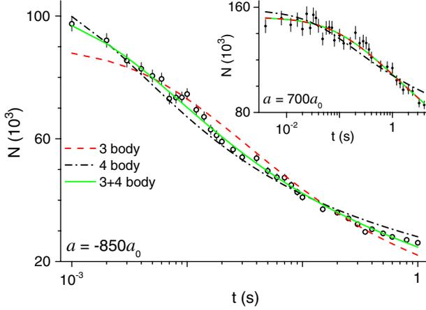
FIG. 3 (color online). Three- vs four-body decay for  $a < 0$  (away from unitarity).  $N$  decay at  $a = -850a_0$  is fitted to a model including both three- and four-body losses (green solid line), as well as to pure three- and four-body models (red dashed and black dot-dashed line, respectively). Inset: For comparison, at  $a = 700a_0$ , the solid green and the dashed red lines are indistinguishable, showing that four-body decay does not play a detectable role.
