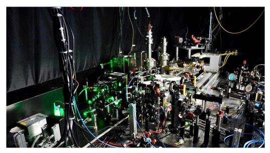
**Fig. 3.1 Photograph of the main experimental apparatus.** The final part of the experiment takes place within the 'science chamber', a glass cell surrounded by the white cross-shaped Feshbach coil holder seen in the middle of the image.
