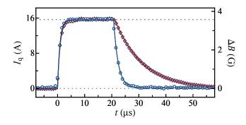
Fig. D.4 Current response of the fast coils used for quenches to unitarity. Here we use an on-resonance hold time  $t_{\rm hold}=20~\mu \rm s$ , and calibrate the field jump magnitude  $\Delta B$  using rf-spectroscopy at unitarity (the conversion as a function of time assumes proportionality with  $I_{\rm q}$ ).
