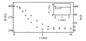
Fig. D.2 Field response following a quench using our primary coils. The quench is initiated at t=0 and the field is measured using rf-spectroscopy as a function of t for two quench protocols depicted in the inset and described in the text.
