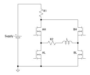
**Fig. D.3 Schematic of the H-bridge circuit used for rapid field switching.** We highlight only the core components of the circuit, which are the power supply, two resistors (R<sub>1</sub> and R<sub>2</sub>), four *n*-channel IXFN48N50 MOSFETS (denoted AH, AL, BH, and BL), and our set of auxiliary coils (denoted L). The circuit is driven using a pair of half-bridge FAN7380 drivers; figure from [86], where additional details are available.
